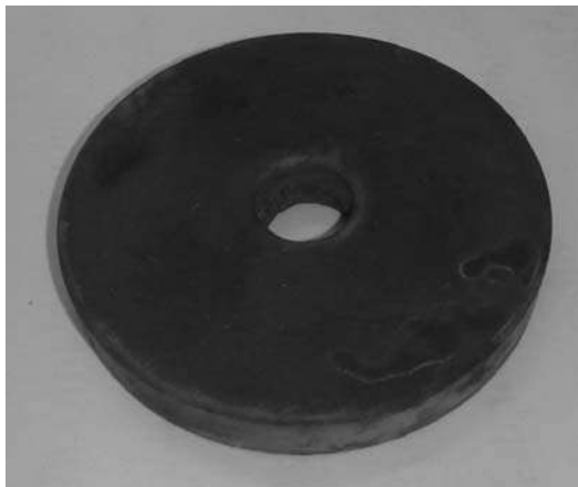
Fig. 2. Mo-Mn metallization layer on ceramic surface
